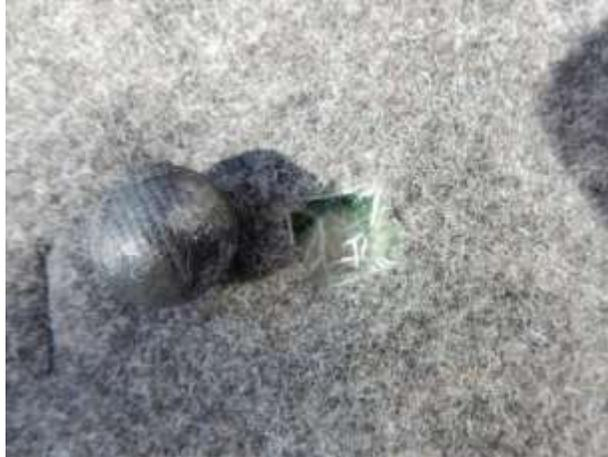
**Figure 8. A fabric impressed .69 diameter ball fired from the British 1756 Long Land Pattern musket with 75 grains of powder at 25 yards. The fabric impressions resulted from passing through the simulated uniform clothing.**
