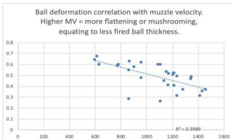
**Figure 22.** Muzzle velocity compared to thickness or flattening of fired balls. The fired ball thickness is in tenths of inches on the left and muzzle velocity is shown on the bottom as feet
