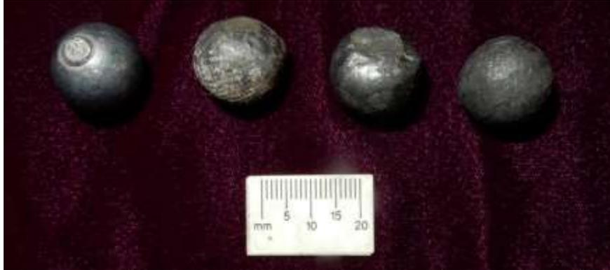
**Figure 14. Unfired. 0.69-inch ball, 0.69 ball fired at 600 f/s that struck ground surface at 100 yards, 0.69 ball fired at 630 f/s that struck a wood table, foam, and ballistic gel at 25 yards and was collected laying on the foam at the back of 32 inches of ballistic gel, and a 0.69 ball fired at 630 f/s that was captured in the ballistic gel at 25 yards after passing through 28 inches of gel. Note fabric impression on second and fourth balls.**
