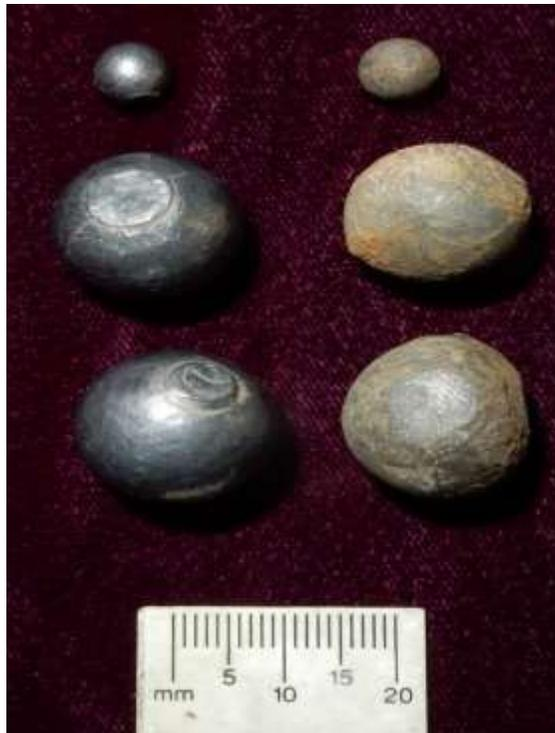
**Figure 16. Top row: Unfired 0.282-inch buckshot and fired 0.282-inch buckshot at 865 f/s. Second row: Unfired 0.626-inch ball and fired 0.626-inch ball at 865 f/s. Third row: Unfired 0.69-inch ball and fired 0.69-inch ball at 870 f/s. Note each recovered in the sand and soil backstop at 100 yards.**
