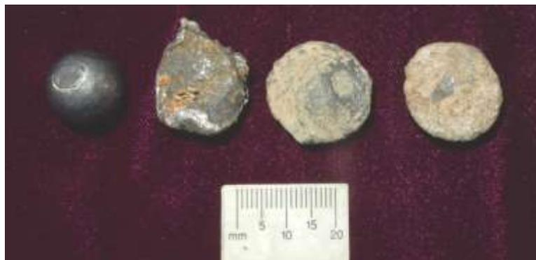
**Figure 21.** Unfired 0.580-inch ball and fired balls, second – fired at 1415 f/s and struck oak palisade paling and found in sand and soil backstop below fence, third – fired at 1435 f/s and found in sand and soil backstop, fourth – fired at 1480 f/s and found in sand and soil backstop. All balls recovered at 100 yards.
