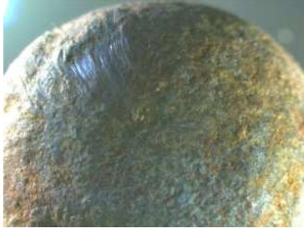
**Figure 25. A 60x magnification of a ball fired in the 1728/41 French musket at 870 f/s that hit the sand backstop. Some slight impact scarring is seen in the upper portion of the image and the fine sand particles impressed on the ball as it struck the backstop.**
