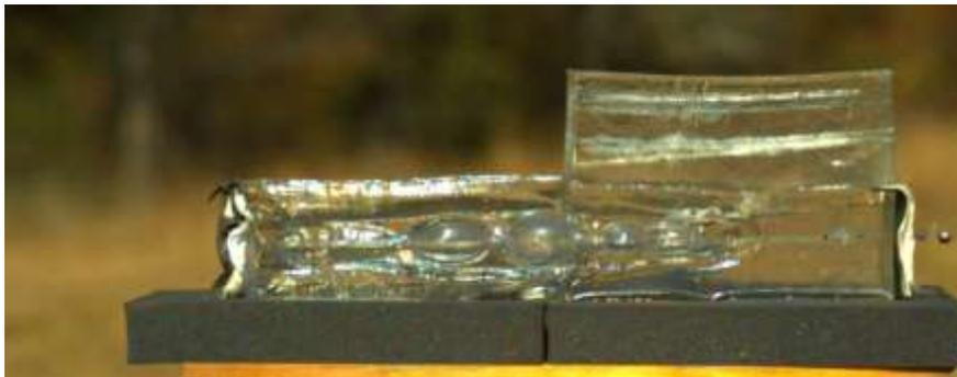
**Figure 7. A .69 diameter ball fired from a British 1756 Long Land Pattern musket exiting 32 inches of gelatin. Note the initial wound cavity, bits of cloth in the wound cavity on the right and a larger piece of cloth exiting the block behind the ball.**
