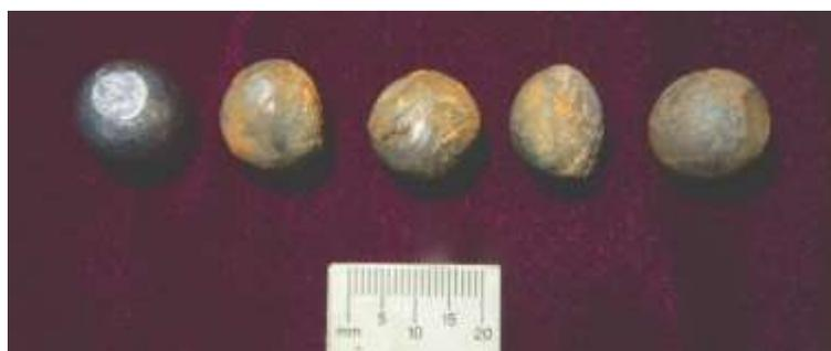
**Figure 17. Unfired 0.626-inch ball, fired balls l to r fired at 905 f/s, 960 f/s, 960 f/s, and 1090 f/s. All balls recovered at 100 yards in sand and soil backstop. Note third ball from the left passed through a pine 4x4 target frame upright and the fourth ball from left also struck the edge of the pine target frame before embedding in the backstop.**
