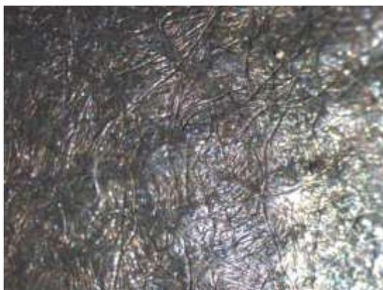
**Figure 24. A 75x magnification of the surface of an unfired lead ball. The lines are a result of the differential cooling at a micro scale of the lead ball when it was cast in a mold. Mold lines and these microscopic cooling lines are indicative of a cast ball. These microscopic cooling lines are largely obscured when a ball is fired.**
