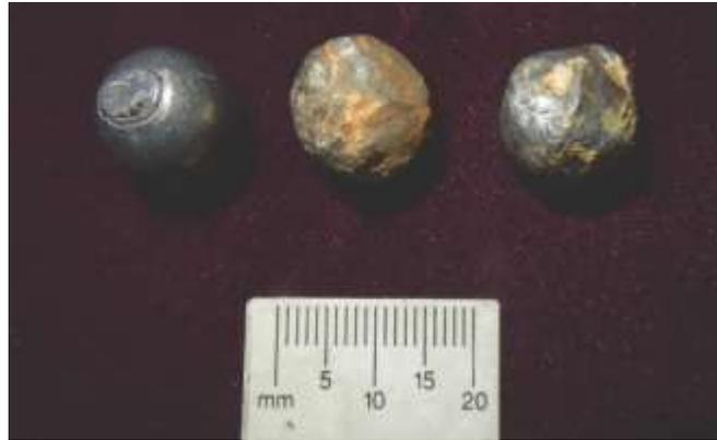
**Figure 20.** Unfired 0.520-inch ball and two fired 0.520 balls, center fired at 1345 f/s and hit pine target frame and right fired at 1350 f/s and hit pine target frame. Both found in sand and soil backstop at 100 yards. Note banding on last ball from being upset in firing from the musket.
