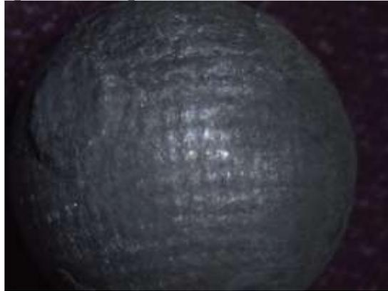
**Figure 26. A 40x magnification of a ball fired from the British 1756 Long Land Pattern musket that passed through the simulated uniform cloth and gelatin blocks. The fabric impressed its weave on the ball providing a textile analyst data for interpretation. The raised circular area on the left of the ball is a sprue from casting the bullet in a mold.**
