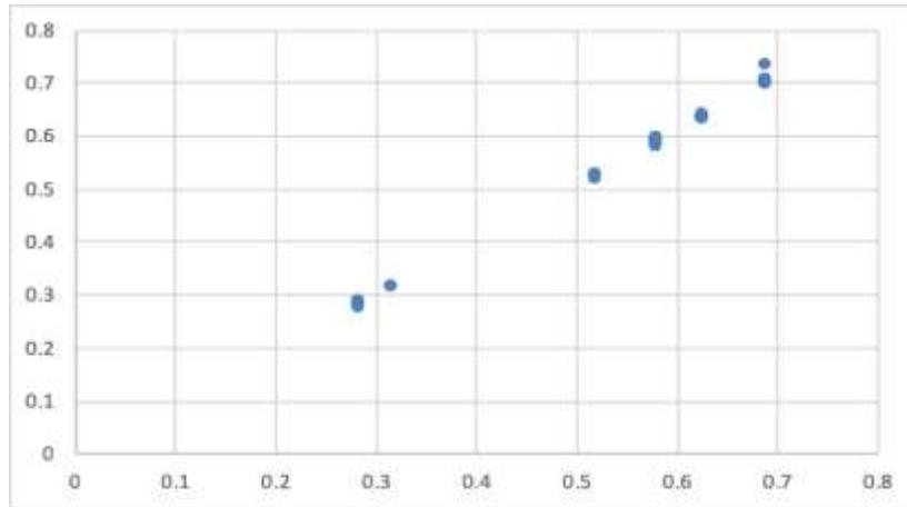
**Figure 12. The measured ball diameter compared to the calculated ball diameter using the Sivilich Formula (2016). The differences are well within one standard deviation with an R value of .998.**
